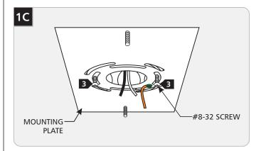
Secure the mounting plate to the junction box with 2 #8-32 screws.
