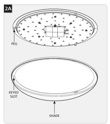
Align the pegs on the mounting plate with the keyed slots on the shade, push the shade onto the pegs, and rotate it to secure in place.
