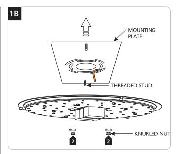
2 Remove the mounting plate from the fixture base by unscrewing the two knurled nuts from the two threaded studs.
