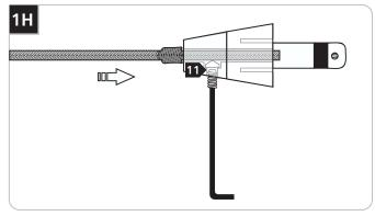
Firmly tighten the set screw on the conical connector.
