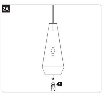
1 Lift the glass shade up to expose the socket.
