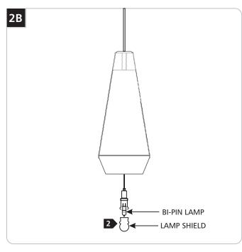
2 Remove the lamp shield and the old lamp.
