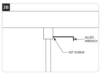
Optional (heads only): To lock the fixture head in a permanent position, tighten the set screw on the fixture Power Jack housing with the provided Allen wrench. This feature is not available on pendants.
