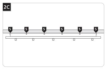
Line up the canopy to the backplate and install all ten (10) button head screws.
