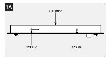
1 Separate the mounting plate from the canopy by removing all four screws.
