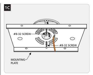
Secure the mounting plate to the electrical box with the two #8-32 screws provided.
