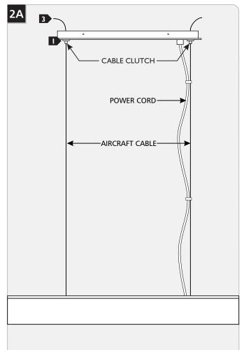
**NOTE:** Make sure to support the fixture while adjusting the aircraft cables. An assistant is recommended to complete the remaining steps.
