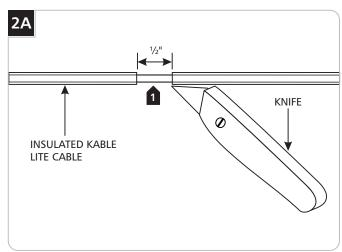
When using insulated Kable Lite cables, remove <sup>1</sup>/<sub>2</sub>" of the insulation from each cable (where the power feed connector is going to be mounted) with a sharp knife. Make sure not to cut or nick the cable.
