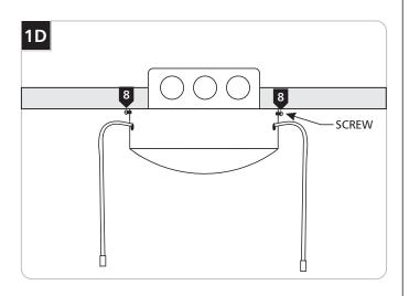
8 Replace the dome cover onto the backplate. Line the dome cover holes up with the backplate holes. Replace and tighten the screws.
