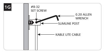
Insert one end of the Kable Lite cable into the slimline post and tighten the #8-32 set screws with the 0.20 Allen wrench to secure the wire. The other end of the cable should be attached to a turnbuckle.
