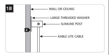
Use the large threaded washer when the Kable Lite cable is attached at an angle to the slimline post.
