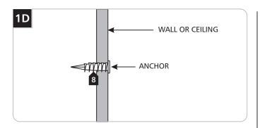
8 Screw the anchors in the rest of the way with a Phillips screwdriver.
