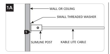
Use the small threaded washer when the Kable Lite cable is attached inline to the slimline post.
