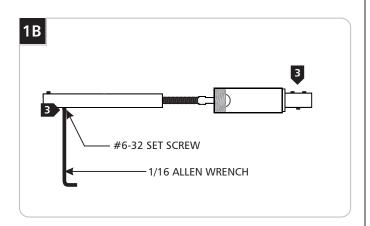
Loosen (Do Not Remove) all five #6-32 set screws with the 1/16 Allen wrench to clear the holes.
