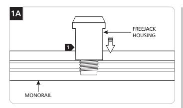
1 From top of the MonoRail place the FreeJack housing onto the MonoRail.
