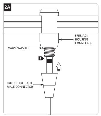
Push and screw the fixture FreeJack male connector all the way into the FreeJack housing connector.
