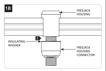
2 From bottom of the MonoRail tighten the FreeJack housing connector to the FreeJack housing.
