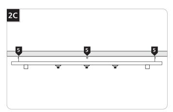
Line up the canopy to the backplate and reinstall all the button head screws.
