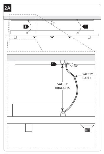
Hook a safety cable through the safety brackets on each end of the canopy and backplate.
