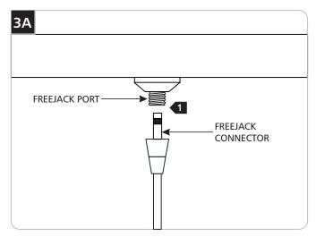
1 Screw a FreeJack connector into each FreeJack port.
