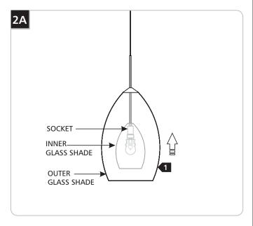
1 Lift the glass shades up to expose the socket.
