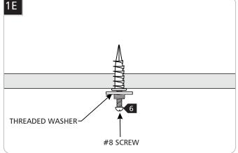
6 Screw the threaded washer onto the anchor with the long #8 screw.
