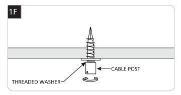
**7** Tightly screw the cable post back onto the threaded washer.
