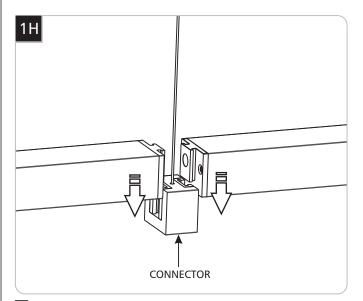
Slid one end of each fixture in to the keyed slot on the connector.
