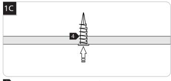
4 Screw the anchor in the rest of the way with a Phillips screwdriver.
