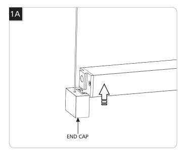
1 Follow the enclosed instructions with the fixture and determine the layout. Make sure the power feed for either of the connecting fixtures is not located above the intersection of the two fixtures.
