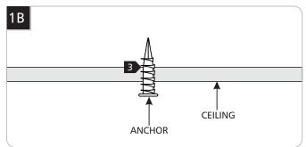
3 Tap the anchor at the marked point into the wall up to the threaded portion with a hammer.
