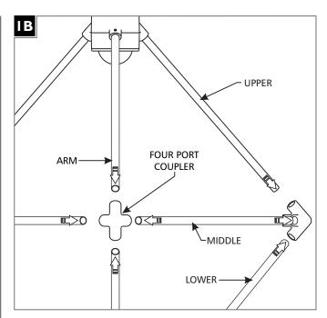
Install the remaining arms by inserting them into the four port couplers. Make sure arms are fully inserted.
