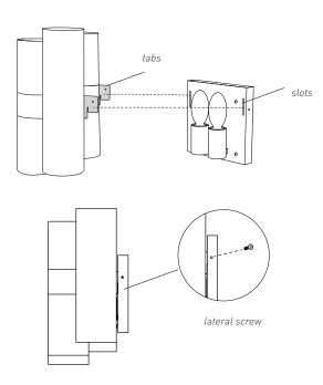
Fit the diffusor tabs in the structure's slots. Secure the the lamp to the wall by using the screws removed in step b.
