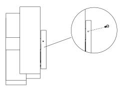
To change bulbs, remove the lateral screws and diffusor. Change bulb or bulbs, and reinstall diffusor and screws.
