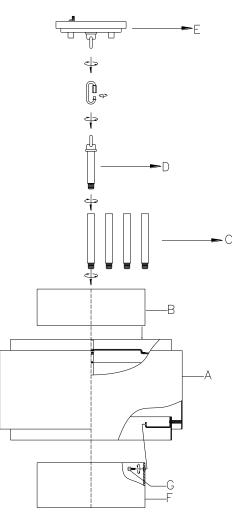
$B \to A \to F \to G \to C \to D \to BULB$
