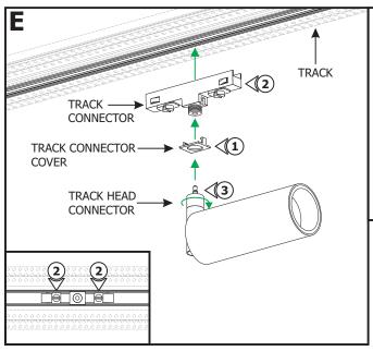
**NOTE:** Omit this section if installing the track head to Vanishing Point Systems.
