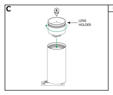
**6:** Screw the lens holder back clockwise to secure in place.
