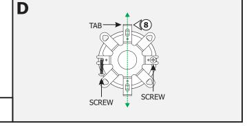
**8:** Align the crossbar tabs <u>vertically</u> and mount the crossbar to the junction box holes with the two #8-32 screws provided.
