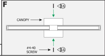
**11:** Place the fixture against the crossbar and secure it with the provided #4-40 screws using a 1/16" Allen wrench.
