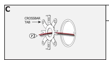
**7:** Feed the wires coming from the DMX controller or dimming module through the center hole of the crossbar. Refer to the instructions provided with the power supply.
