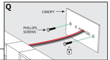
**5:** Place the canopy onto the junction box. Secure it to the junction box with the two Phillips screws provided.
