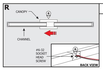
**6:** Insert the socket head cap screws into the opening of the canopy, then slide the channel sideways to lock in place.
