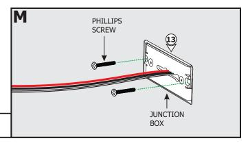
**13:** Place the mounting plate into the junction box. Secure it with the two Phillips screws.
