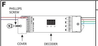
**11:** Loosen the Phillips screw on the input side of the decoder to remove the cover.
