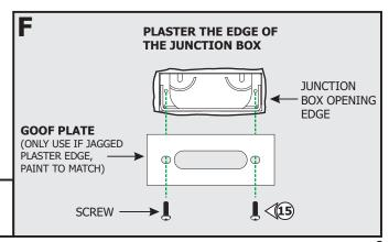
**15: Optional:** Use the Goof Plate if the junction box opening has imperfection/ jagged edges. Install the provided goof plate (paint to match prior) with the two screws.
