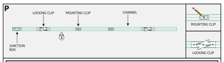
NOTE: Clips must be leveled and centered. They must be installed maximum 24" from each other.
