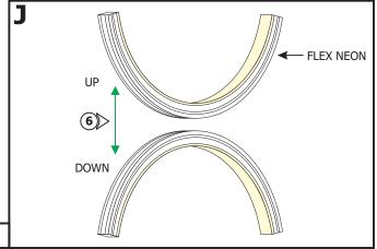
**6:** If necessary, bend the Flex Neon **ONLY** up and down.
