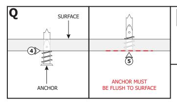
**NOTE:** Steps 4 and 5 are for drywall mounting. Omit these steps if mounting to a wood surface directly.
