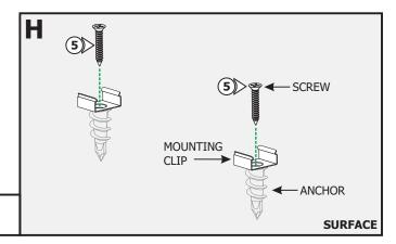
**5:** Line up the mounting clips to the anchors and secure it to the anchors by tightening the #8-32 screw to each clip.
