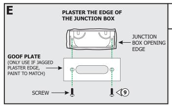
**9: Optional:** Use the Goof Plate if the junction box opening has imperfection/ jagged edges. Install the provided goof plate (paint to match prior) with the two screws.
