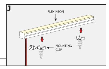
7: Insert the Flex Neon into each mounting clip.
