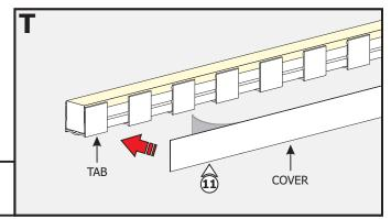
**11:** Remove the backing from the channel cover. Firmly press down on the Flexible Aluminum Channel tabs while removing the rest of the backing.
