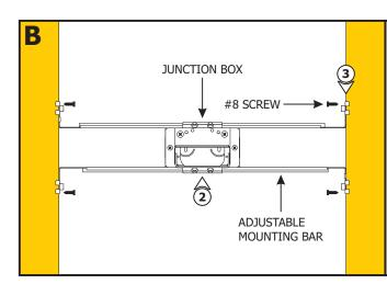
**NOTE:** The adjustable mounting bars mount to studs/joists that are spaced 15"-24" apart. If the span needs to be shorter than 15", then break the bar arms from dedicated lines.
