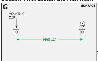
**NOTE:** If using 1RE Junction Box, the Flex Neon must pass through the center of the junction box.
