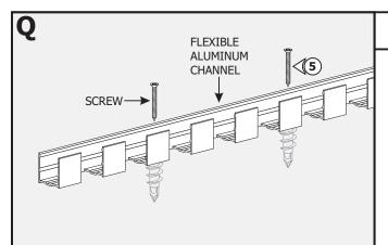
5: Secure the Flexible Aluminum Channel to the anchors using screws.
