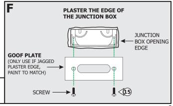
**15: Optional:** Use the Goof Plate if the junction box opening has imperfection/ jagged edges. Install the provided goof plate (paint to match prior) with the two screws.
