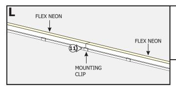
**11:** For seamless continuous runs, place a second seamless Flex Neon at one end of the first Flex Neon. Ensure that a mounting clip is in the center where the fixtures meet together.
