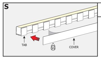
**11:** Remove the backing from the channel cover. Firmly press down on the Flexible Aluminum Channel tabs while removing the rest of the backing.
