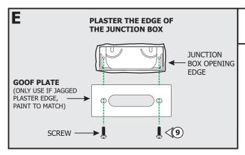
**9: Optional:** Use the Goof Plate if the junction box opening has imperfection/ jagged edges. Install the provided goof plate (paint to match prior) with the two screws.
