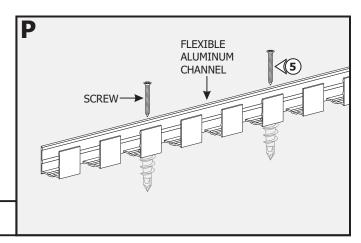
**5:** Secure the Flexible Aluminum Channel to the anchors using screws.
