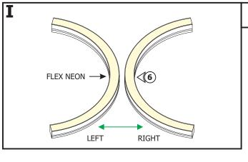
**6:** If necessary, bend the Flex Neon **ONLY** right to left or left to right.
