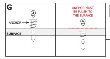
**NOTE:** Steps 3 and 4 are for drywall mounting. Omit these steps if mounting to a wood surface directly.
