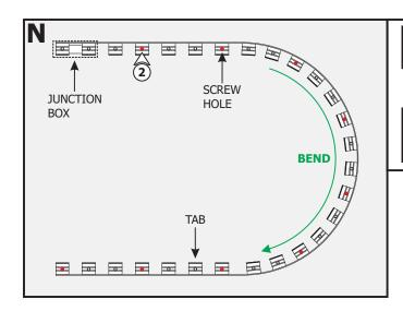
**NOTE:** If using 1RE Junction Box, the channel must pass through the center of the junction box.
