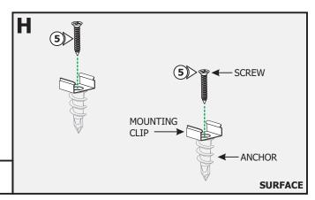
**5:** Line up the mounting clips to the anchors and secure it to the anchors by tightening the #8-32 screw to each clip.
