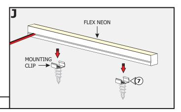
7: Insert the Flex Neon into each mounting clip.
