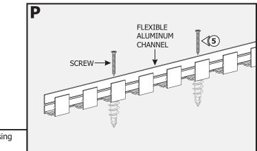
**5:** Secure the Flexible Aluminum Channel to the anchors using screws.
