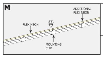
**11:** For seamless continuous runs, place a second seamless Flex Neon at one end of the first Flex Neon. Ensure that a mounting clip is in the center where the fixtures meet together.
