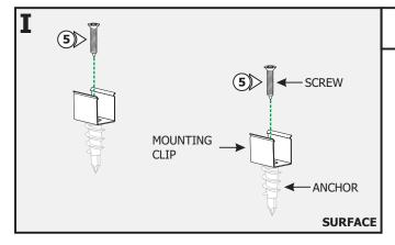
**5:** Line up the mounting clips to the anchors and secure it to the anchors by tightening the two #8-32 screws to each clip.
