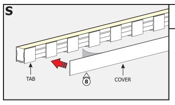
8: Remove the backing from the channel cover. Firmly press down on the Flexible Aluminum Channel tabs while removing the rest of the backing.
