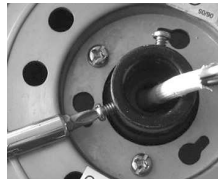
loosen set screws on coupler
