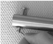
remove stopper pin, cotter pin and washer
