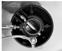
remove half-ball and stopper pin
