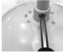
reinstall and tighten stopper screw
