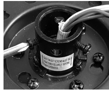
loosen screws on coupler
