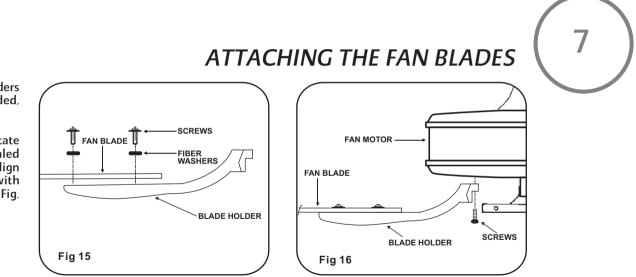
Step 1. Attach the fan blades to the blade holders using the screws and fiber washers provided, tighten screws securely. (Fig. 15)
