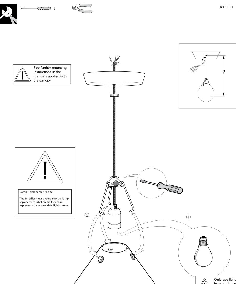
Only use light source in accordance to the lamp replacement label on the luminaire
