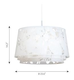
Description The fixture emits diffused light directed primarily downwards. The patterns on the three laser cut acrylic shades have been carefully staggered with the aim of eliminating unpleasant glare from the light source. The patterns differ between the shades, resulting in different perceptions of light and shadow depending on the viewing angle.
