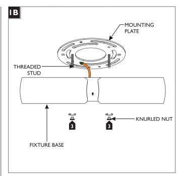
Remove the mounting plate from the fixture base by unscrewing the two knurled nuts from the two threaded studs.
