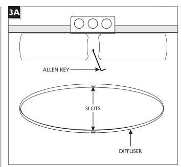
Install the diffuser by placing a diffuser slot onto the unloosened set screw, then align the other slot with the loosened set screw, and re-tighten the set screw using the provided Allen key.
