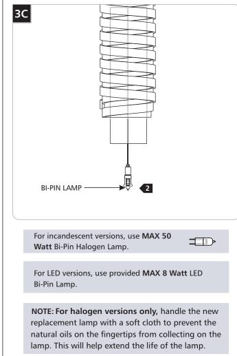
Gently insert the new lamp into the socket.
