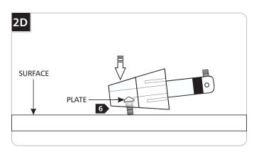
6 Tap the conical connector on a hard surface with the set screw facing down, so the plate inside drops into place.
