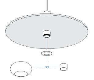
To install acoustic panel, insert light fixture through the center hole in the acoustic panel first, then sandwich the provided 2" acrylic support plate in between and tighten 1" tube from below. Let the acoustic panel rest on the 2" acrylic support plate. You may optionally substitute the 1" tube with a glass shade.
