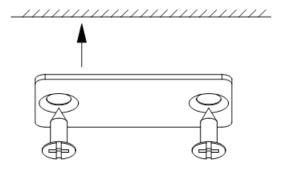
4. The back of the remote control magnetically mounts to the wall bracket.
