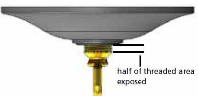
Drawing 2 – Canopy Adjustment
