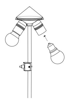
Remove top to install the shade. Turn top counter clockwise to loosen.
