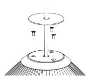
Put the top hat on the lantern and screw the top hanger with the rubber disc through the hat and into the lantern.
