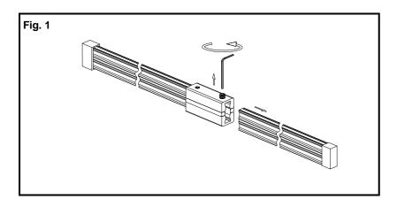
1. Unscrew the Allen Set Screws using the Allen Wrench provided.
