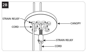
2 Feed a fixture cord through each strain relief.
