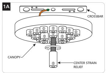
Remove the crossbar from the canopy by completely unscrewing the center strain relief.
