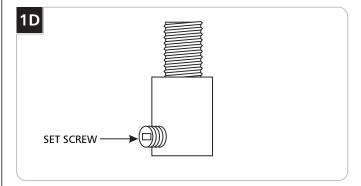
6 Loosen (Do Not Remove) the set screw on each strain relief.
