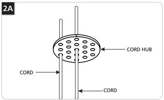
1 Feed a fixture cord through each hole in the cord hub.
