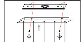
**Step.3:** Tighten screws on the sides of the canopy (C) to secure the fixture.
