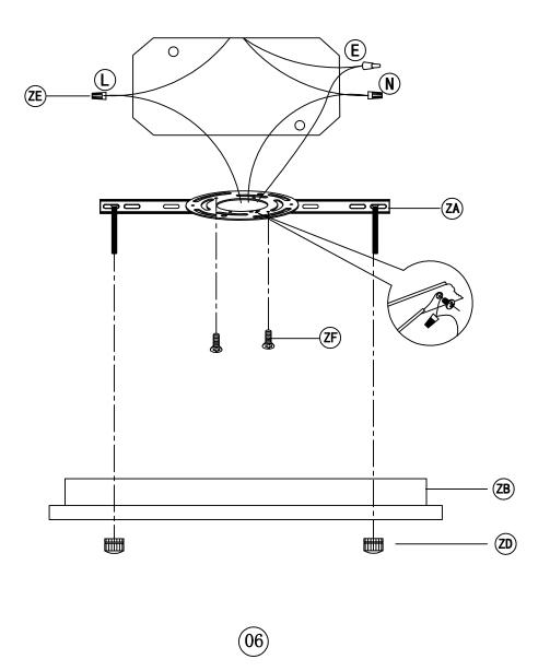
IMPORTANT: Test sockets with bulb before dressing the fixture.
