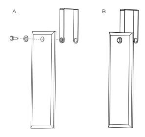
4 . Install the glass onto the bracket as shown.
