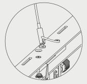
2. Fix the mounting plate to the ceiling. Ensure that suitable screws are being used for the surface that you are mounting to (not supplied).
