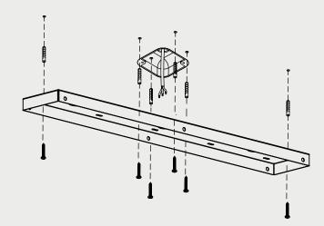
**3**. Raise the pendant towards the ceiling and make the electrical connection, threading the cable through the center of the ceiling rose.
