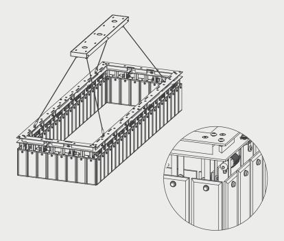
Tilt inner ring and lift it up through the middle of the support beam then lower it down to locate the fixing brackets onto the locating holes in support beam top.
