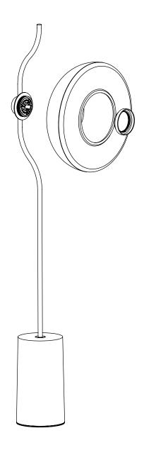
**3**. Screw the diffuser (D) into the centre of the body.
