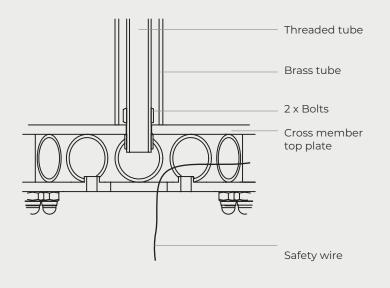
Insert the safety wire (already attached to the cross-member) through the drop rod and ceiling rose.
