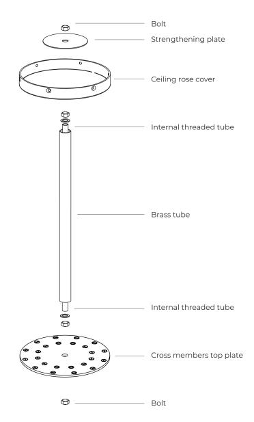
Remove the first M13 nut from the bottom of the drop rod (leave the second nut) and attach the drop rod to the top plate of the cross member, replacing the nut and tightly securing (socket set required).
