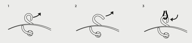
**9**. Hang the remaining disk from the threaded brass ring at the bottom of the pendant, as shown in the diagram.
