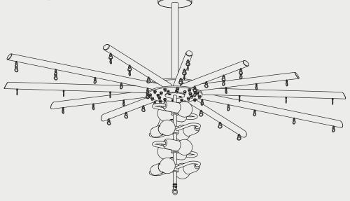
**6**. Fit the bottom glass disc to the lamp holder assembly using the threaded ring and rubber washers each side of the glass (as shown in diagram).
