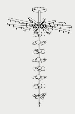
6. Fit the bottom glass disc to the S-arm assembly using the threaded ring and rubber washers each side of the glass (as shown in diagram).
