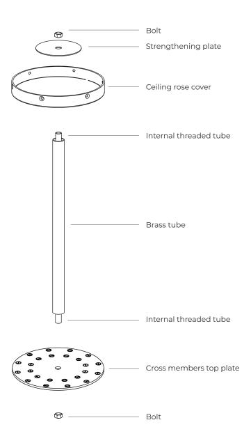
Use bolt (provided) to assemble the drop rod (threaded tube) with the top plate of the cross member (socket set required).
