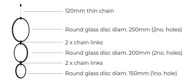
8. Hang the 'central glass chain' disks from the threaded brass ring at the bottom of the pendant, as shown in the diagram.
