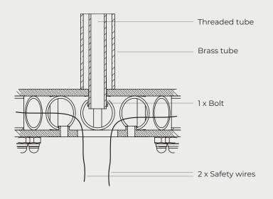
2. Insert the 2 x safety wires (already attached to the cross-member) through the drop-rod and ceiling cover plate.
