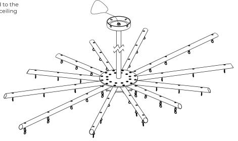
3. Insert the power cable through the cross member and drop rod, and pull through and out of the ceiling cover box.
