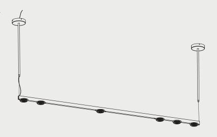
Raise the pendant and make the electrical connections ensuring all wires are colour matched and the pendant is earthed correctly on one of the drop rods.
