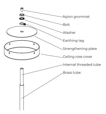
Mark on the ceiling the location for the 2x ceiling roses. The center of these needs to be 1680mm (66.2 inches) appart.
