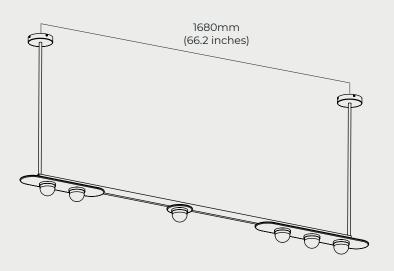
2. Fix both mounting plates to the ceiling. Ensure that suitable screws are being used for the surface that you are mounting to (not supplied).
