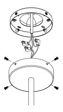
Fit the back glass onto the body by screwing on the dome glass.
