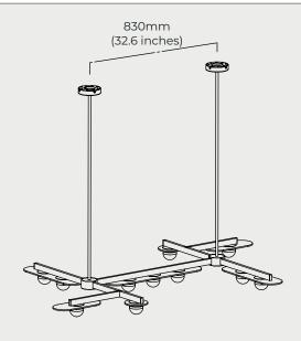
2. Fix both mounting plates to the ceiling. Ensure that suitable screws are being used for the surface that you are mounting to (not supplied).
