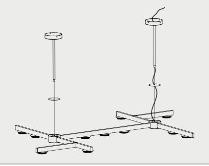
Raise the pendant and make the electrical connections ensuring all wires are colour matched and the pendant is earthed correctly on one of the drop rods.
